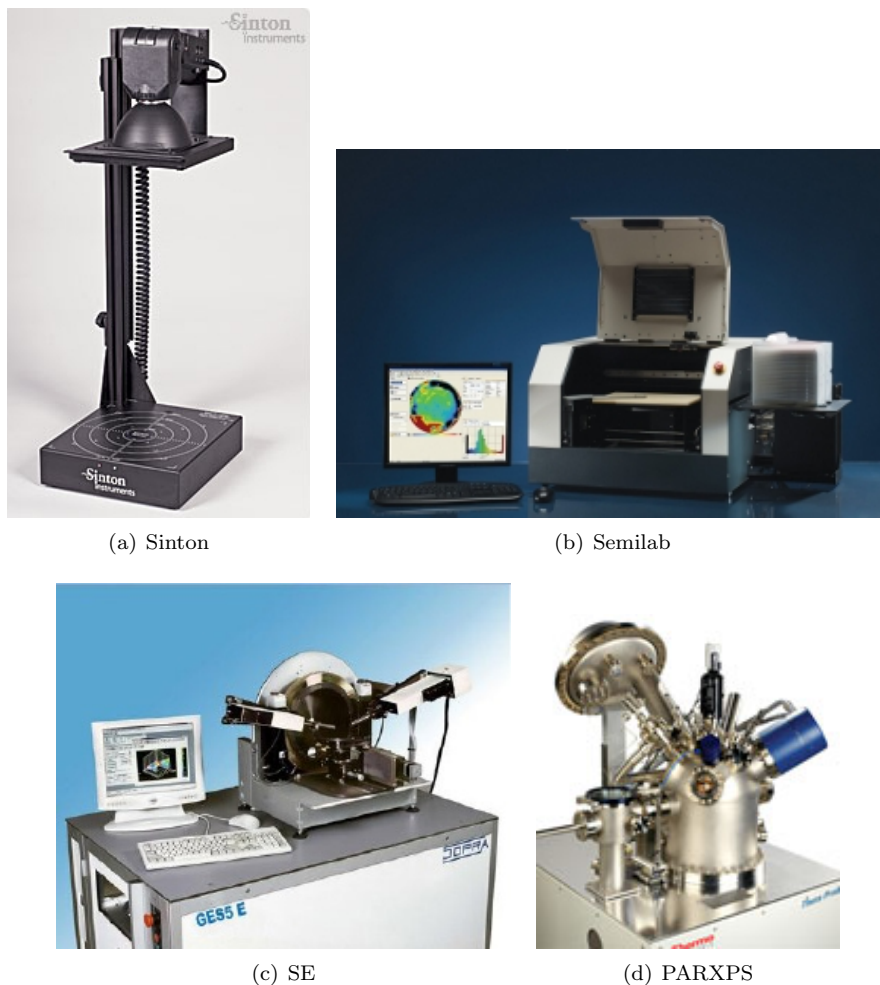
Figure 3.4: Measurement devices: a) Sinton lifetime tool b) Semilab lifetime tool c) Sopra spectroscopic ellipsometer d) Thermo Scientific parallel angle-resolved x-ray photoelectron spectroscopy. Pictures are downloaded from the company webpages.
