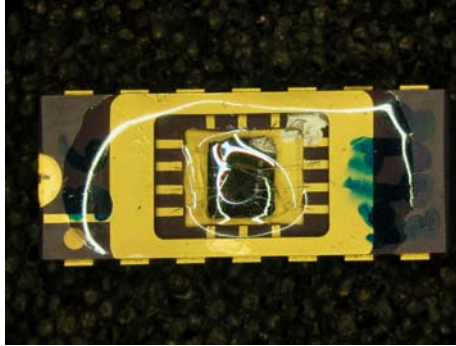
Figure 2.7: Photograph of a packaged SiNW sample: The sample is glued on a chip carrier and the nanowires are bonded to the pins of the carrier. In order to allow measurements in liquids, all metallic parts are sealed with an insulating transparent epoxy.
