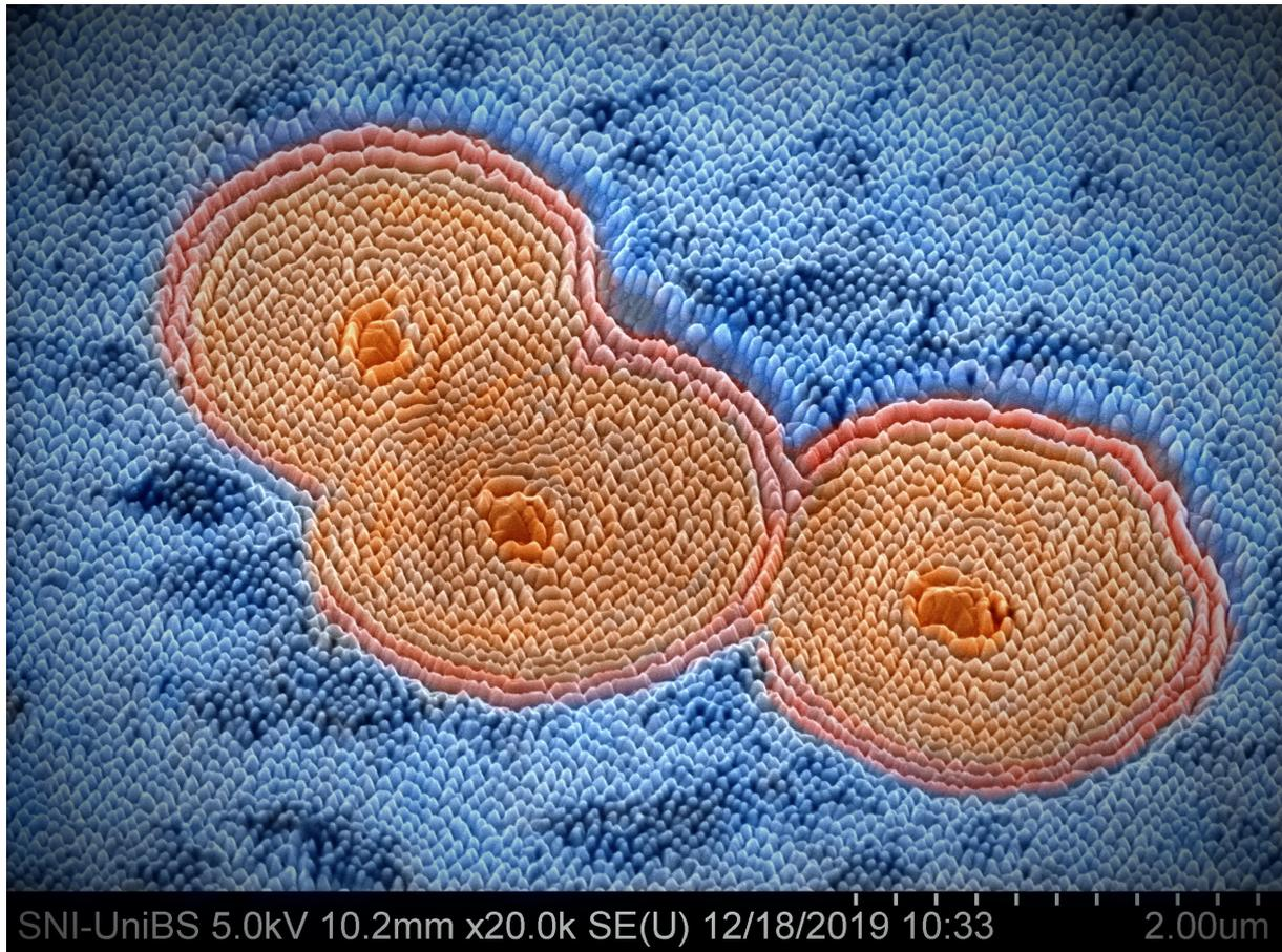
*This image is a top-view of a single-crystal rhodium imaged by a Hitachi S4800. The exposure of the Rh surface to Ar<sup>+</sup> leads to the appearance of ripples that propagate outwards, eventually leading to coalescence.*
