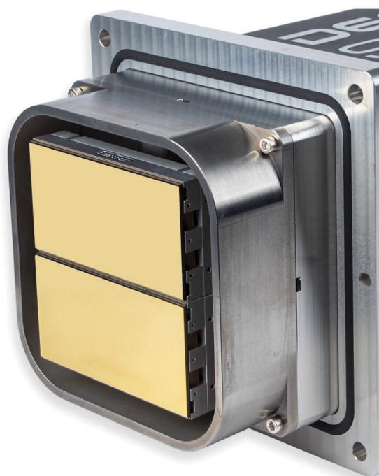
Fig. 3: Prototype dual-module Dectris detector for future applications in cryo electron tomography of biological specimens.
