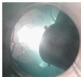
Fig. 3: Confined He ion beam produced by a HiPIMS excited UBM sputtering technique.
