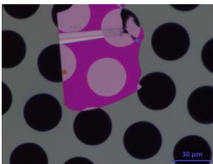
Fig. 4: Optical microscope image of an hBN drum resonator on a custom Norcada SiN membrane. More recently, we have integrated these devices into our cavity to characterize their mechanical properties and the resulting optomechanical interaction.
