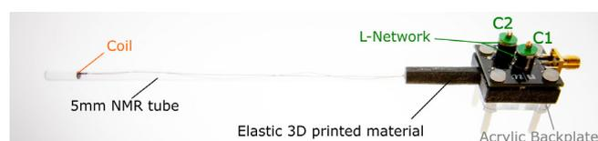
Fig. 4 DeePest NMR probe featuring the inserted coil and the matching/tuning circuit. The DeePest electronics is connected to this probe.
