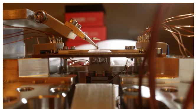
Fig. 2 Side view photograph of the ion trap corresponding to the schematic in figure 1. The nanowire holder can be seen between the electrodes in the trap center.
